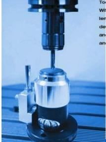
Toolsetter 35.10-TS establishes tool geometries on the machine. With its precise measuring mechanism, it reliably determines length and radius of the tool, measures single edged cutters and detects broken tools. Measuring can be made both statically and dynamically. It has been designed for use on milling machines and machining centres.
